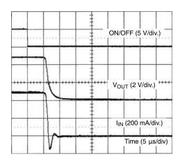
SiP4280-1 Turn-Off (V<sub>IN</sub> = 5 V, R<sub>LOAD</sub> = 10  $\Omega$ )
