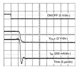
SiP4280-1 Turn-Off (V<sub>IN</sub> = 3 V,  $R_{LOAD}$  = 6  $\Omega$ )
