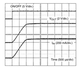
SiP4280-1 Turn-On (V<sub>IN</sub> = 5 V, R<sub>LOAD</sub> = 10  $\Omega$ )
