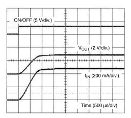
SiP4280-1 Turn-On (V<sub>IN</sub> = 3 V, R<sub>LOAD</sub> = 6  $\Omega$ )
